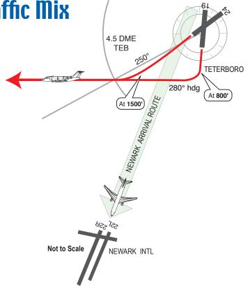
2.8 DME instead of the required 4.5 DME for climbing to 2,000 feet MSL. I instructed the SIC to descend back to 1,500 feet MSL until the 4.5 DME then climb to 2,000 feet. ATC called and indicated that we climbed too early. The departure was properly briefed.
