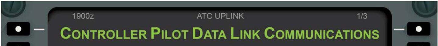
Controller Pilot Data Link Communication Departure Clearance Services (CPDLC-DCL) is one segment of the Future Air Navigation System (FANS) that has been recently implemented in the contiguous 48 states at local Tower Data Link Service (TDLS) equipped facilities to deliver departure clearances and revised departure clearances prior to takeoff.
